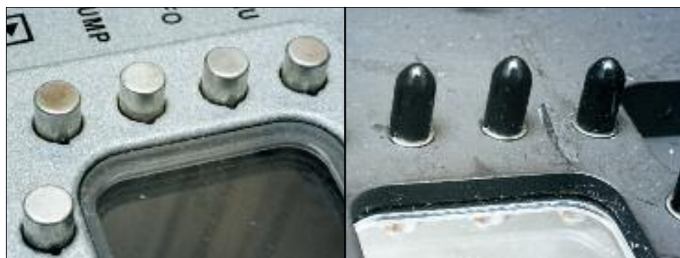
Modern digital housings are studded with a plethora of control knobs and rods (left). They are spring loaded and held in with small stainless steel circlips (right). I would have to remove the black soft plastic sleeves first then gently pry off the circlips with a small screw driver. Be careful that you do not launch them into space as they are easy to lose, along with the internal springs and any washers that may be in there.
