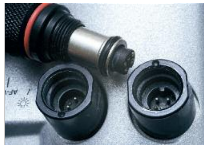
The long body of Nikonos strobe connections add leverage which can deform or nick the small O-ring. If in doubt, replace them often. You cannot see the seal in a bulkhead connection so a new O-ring and gentle insertion, feeling for any catching or pinching, is the way to go. Be sure to insert the strobe end straight into the bulkhead connector, as forcing it in at an angle will damage the O-ring.
