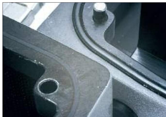
A faint mark is left on the sealing surface of the housing back. You can check it for any signs of breaks which may be caused by hairs, fluff or a pinched O-ring. Perspex housings may allow you to view the O-ring while sealed so that you can see any breaks or gaps.
