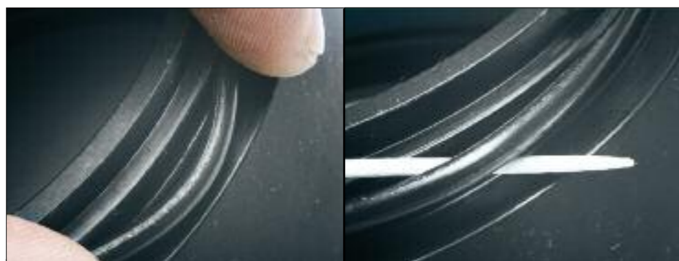
Before you remove an O-ring check the manufacturer's housing manual. Some, such as the superbly crafted Nexus housings, demand that you never remove the main O-ring seal. If that's the case, just wipe the O-ring with your clean lint-free cloth. For other O-rings, you can gently pinch with your fingertip pads (left) or use a non-metallic object, such as this wooden tooth pick (right), to lift it out of the groove. To avoid scratching the groove/channel you may want to use the blunt type of toothpicks, not the pointed variety shown.
