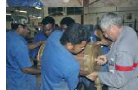
Seine double wheel pieces are assembled after an electrolytic treatment. (Pierre Larue FMC); La Seine twin steering wheel is drawn by computer assistance. (Pierre Larue FMC); Inside technical high school work shop, teacher Marc Jeandel, runs with his pupils La Seine twin steering wheel restoration, using pieces of kohu (local wood). (Luc Faucompré FMC); Ten kohu elements are assembled on each steering wheel. (Luc Faucompré FMC); Positioning the axis through the drum on the original mounts. (Pierre Larue FMC).
